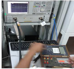
Fig. 4 VNA Measurement Setup
